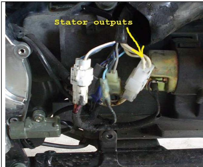
Look for the wire bundle that comes out of the engine. There will be 2 groups of wires in this bundle. One will have 2 wires going to a connector, the other will have 3 wires going to a connector. You want the one with 3 white wires going to it.
