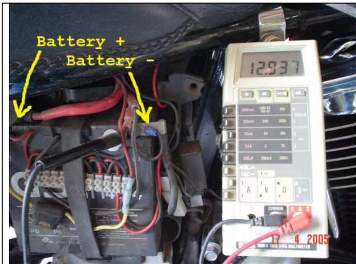
Measure the voltage (DC) across the battery. It should read about 12.4 – 12.9 volts.
